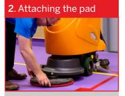
Attach the red pad underneath the scrubbing/suction machine.
